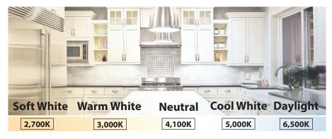
Color temperature describes the light appearance of a light bulb and is measured in Kelvin (K).
