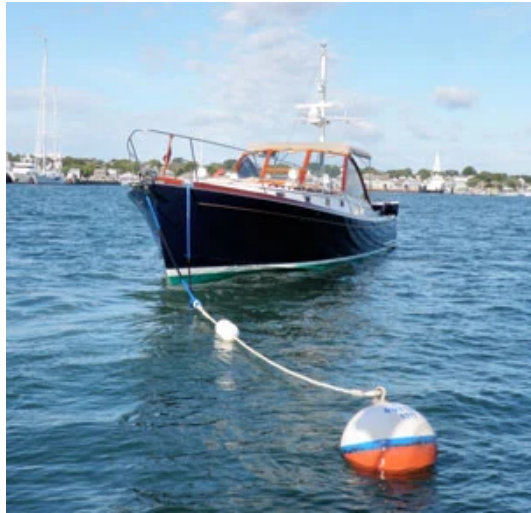
This powerboat is moored through both bow chocks with two of New England Ropes' Cyclone Mooring Pendants . The bottom white section of the pendant is traditional three-strand nylon.
