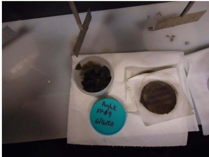
**Sample B-6, 500 ppm polymer 626, 1 hour @ 125psi Filter Cake and filter cloth (above) and filtrate (left).**
