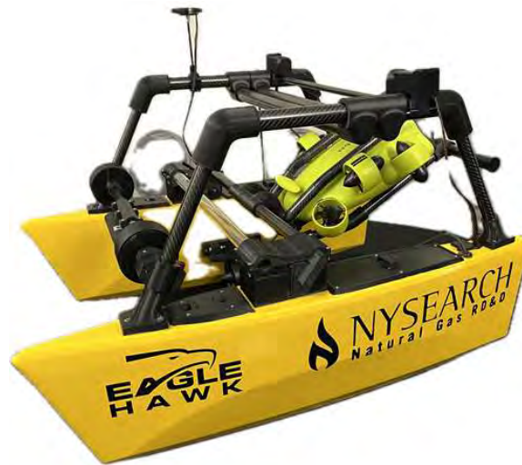
Figure 47: Aquatic Drones Perform Inspections of Submerged Pipelines
